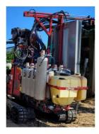
Motorized vineyard sprayer : soil protecting & drift reducing crawlermounted tunnel sprayer
